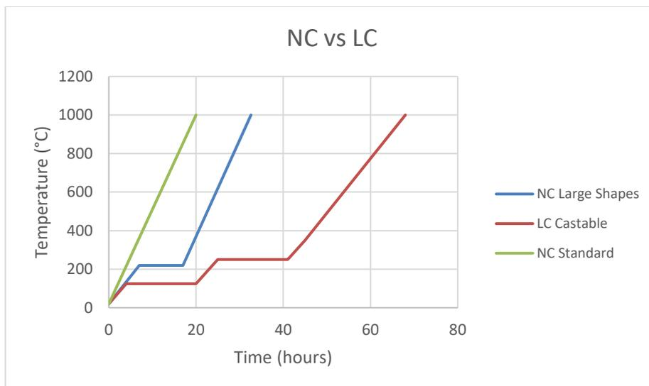
From the dry-out profile shown above it is clear that substantial time savings can be achieved in installations using NC (Non-cement) castable when compared to LC (Low Cement) Castable. Further to this the NC standard **dry out profile is much less demanding** technically than the multistep profile of LC (Low cement).
