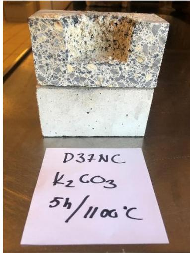
The strength of the silica gel bonding system also means that the **strength of D37NC rises with increased temperature**. The high strength bonds also help to give D37NC a **good abrasion index** measured at only 3,1cm<sup>3</sup> loss at 90° according to ASTM C704.
