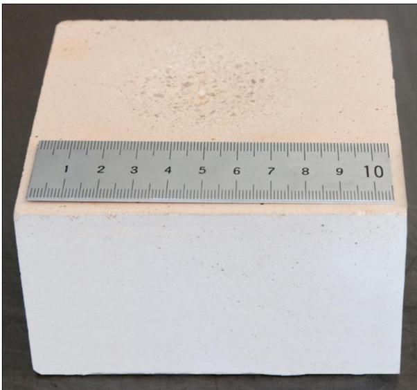
At HASLE we measure wear resistance as abrasion loss at 1000°C according to ASTM C704, where SiC particles are blown against precast samples. Measuring at high temperature simulates the performance during operation better than if measured at room temperature.
