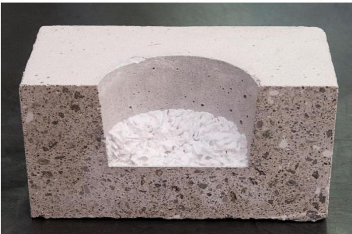
This picture shows the result of a standard alkali-test of D39A-EF with K<sub>2</sub>CO<sub>3</sub> at 1100°C according to EN/TS 15418.
