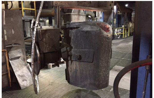
Transport ladle lined with HASLE D1700A
