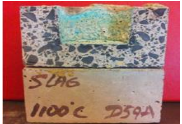
Slag test result, HASLE D59A at 1100 degrees Celcius
