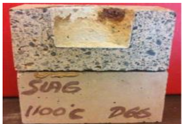
Slag test result, HASLE D66 at 1100 degrees Celcius
