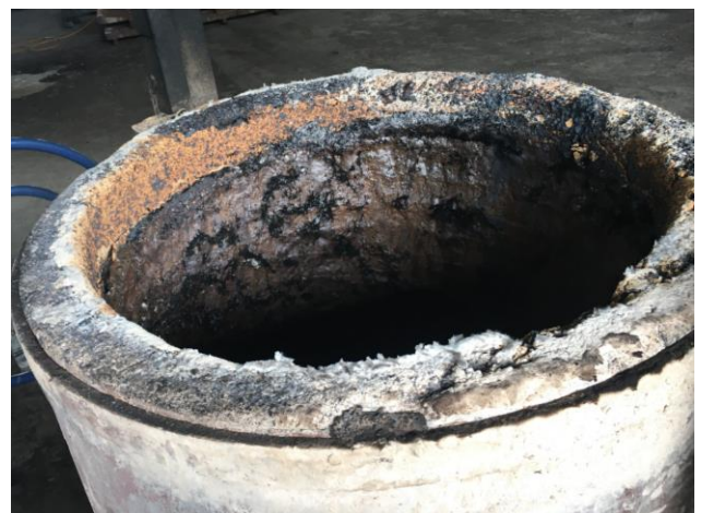
Ladle after 195 heats and still running
