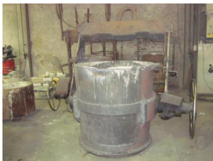
Big ladle for grey iron lined with HASLE D1700A
