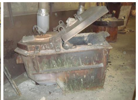
Tundish lined with HASLE D1700A
