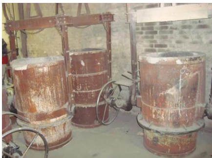
1T ladles for cast iron lined with HASLE D1700A
