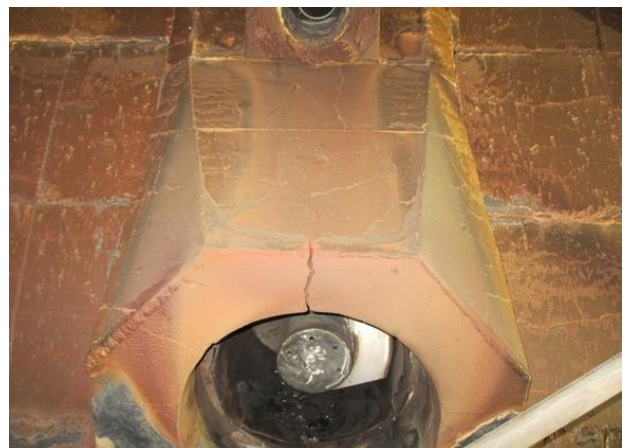
Feeder Burner after 12 months
