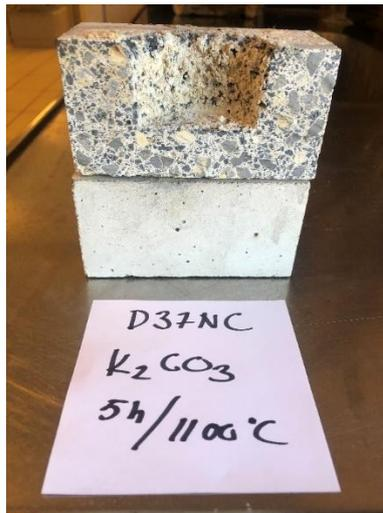
The strength of the silica gel bonding system also means that the **strength of D37NC SC rises with increased temperature**. The high strength bonds also help to give D37NC SC a **good abrasion index** measured at only 3,1cm<sup>3</sup> loss at 90° according to ASTM C704.
