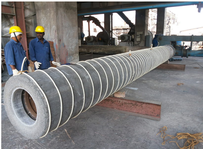
In the process of setting up a burner pipe for controlled preheating, attaching the heating coils.
