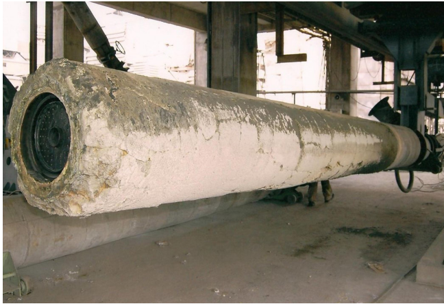
The burner pipe after around 12 months of operation at Ramco Cement's Jayanthipuram plant.
