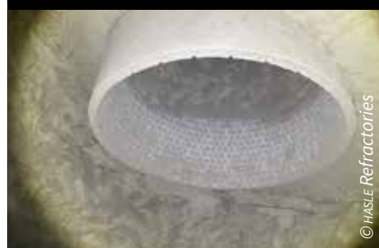
The CVF in the second-lowest stage cyclone after one year of operation at the German cement plant
