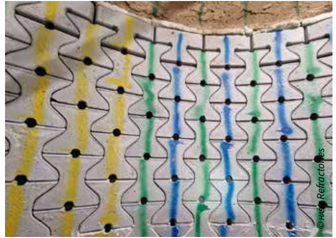
The third-generation Ceramic Vortex Finder fully assembled in one of the lowest stage cyclones at the German cement plant
