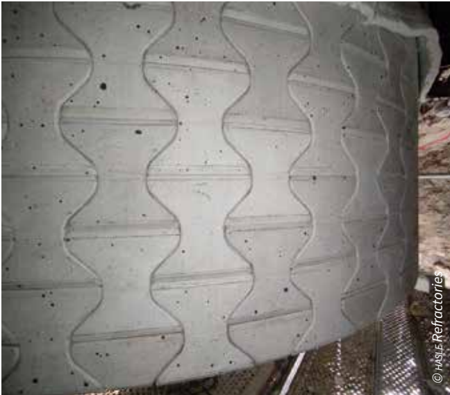
The third-generation Ceramic Vortex Finder fully assembled in one of the lowest stage cyclones at the German cement plant
